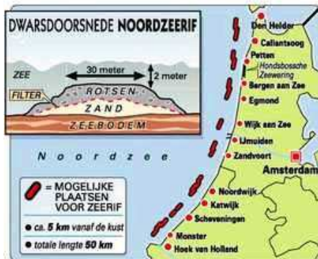
Figure 62: Possible design for artificial reefs protecting the Holland coast [WINN, 2008].
