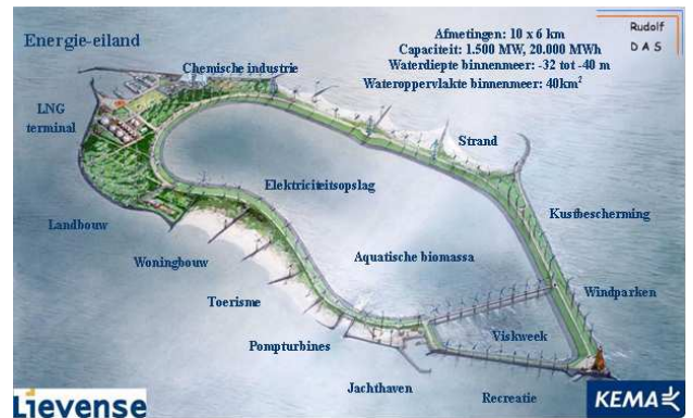
Figure 61: The energy-island design of Lieveense, combining hydropower generation and other land-use functions in one island [Lieveense, 2008].
