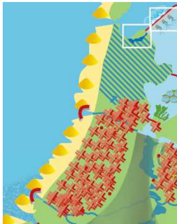
Figure 69: Witteveen+Bos foresees a seaward extension of the Dutch coast in its Deltaplan 2008-2100. New dunes should be created in front of the present coastline [Witteveen+Bos, 2008].
