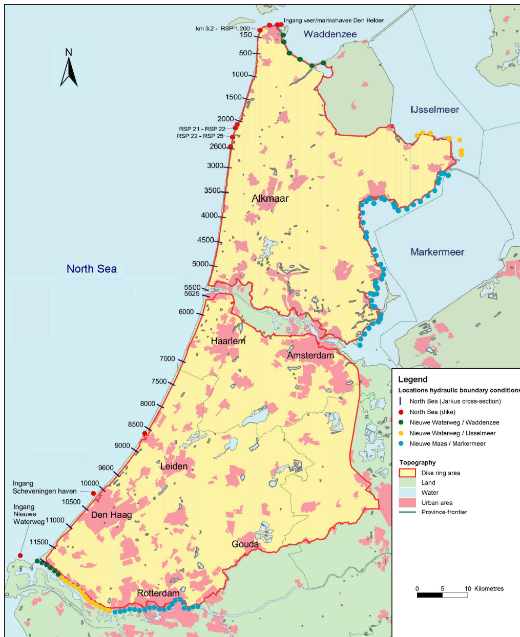
Figure 52: Locations of the Jarkus section lines along the Holland coast. The upper part of the study area is dike ring 13, the lower part is dike ring 14. The red dots along the coast represent the locations of (small) dikes [Min V&W, 2007].
