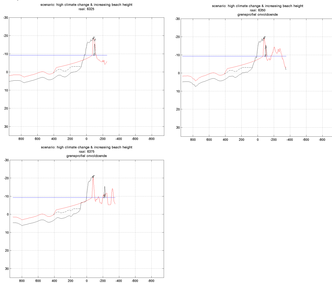
Figure 55: Erosion calculation results for the high climate change scenario; cross-sections 6325, 6350 and 6375.
