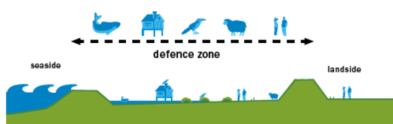
Figure 77: The ComCoast principle: changing single line defences to wider defence zones with opportunities for nature and recreation [ComCoast, 2007].
