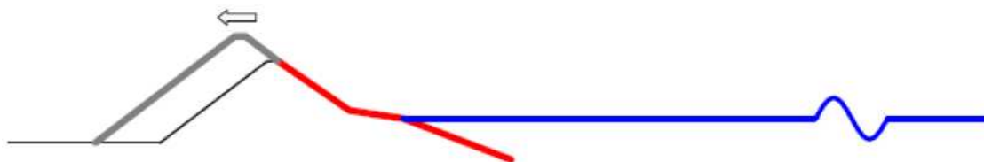
Figure 96: Schematic representation of dike heightening and the induced landward extension of the inner slope of the dike [Hoogheemraadschap Hollands Noorderkwartier, 2008].
