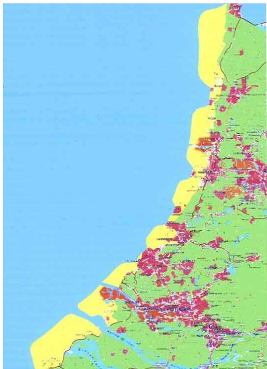
Figure 68: Extension of the coastal defences according to Bos, also called the 'Bos-variant'. Dunes are significantly extended in seaward direction accommodating both nature and economic values [Bos, 2001].
